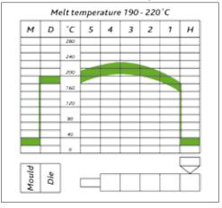
Cooling water (Chill roll) 15-30°C Cooling water (Water bath) 15-40°C Cooling water (Monofilaments) 60°C
